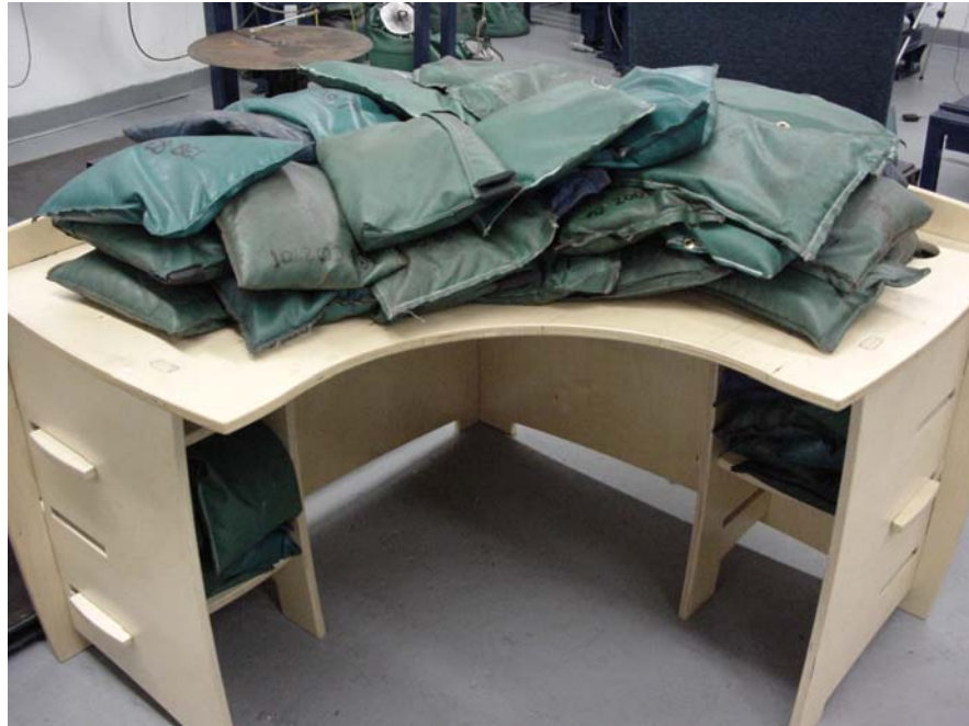
Figure 1. Distributed Horizontal Surface Static Load Procedure 1000 lb. Load
